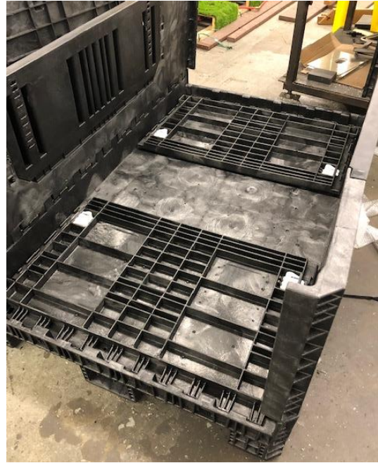
Photo 9 – Second Collapsible Side
